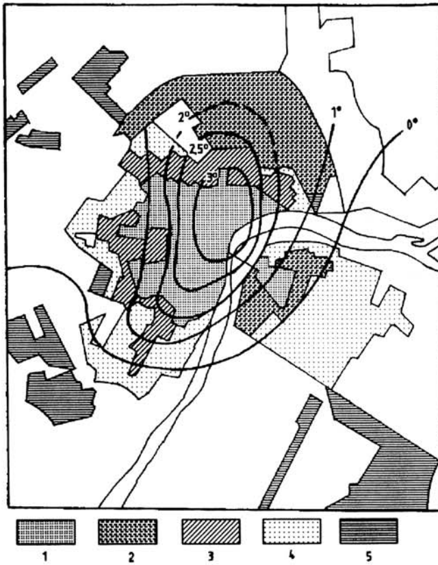
Fig. 6 The isotherms of daily mean minimum temperature difference in winter and morphological map of Szeged: 1 - big town type, 2 - concrete housing estate type, 3 - small town type, 4 - suburb type, 5 - village type (after Zsiga, 1983)
